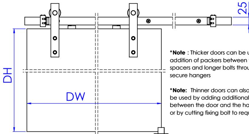
\*Note : Thicker doors can be used with the addition of packers between the wall and wall spacers and longer bolts through the doors to secure hangers
